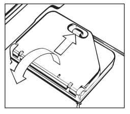
■ Press the opening catch on the container (see arrow) forwards. The flap will spring open. (The flap is always open at the end of a program).
